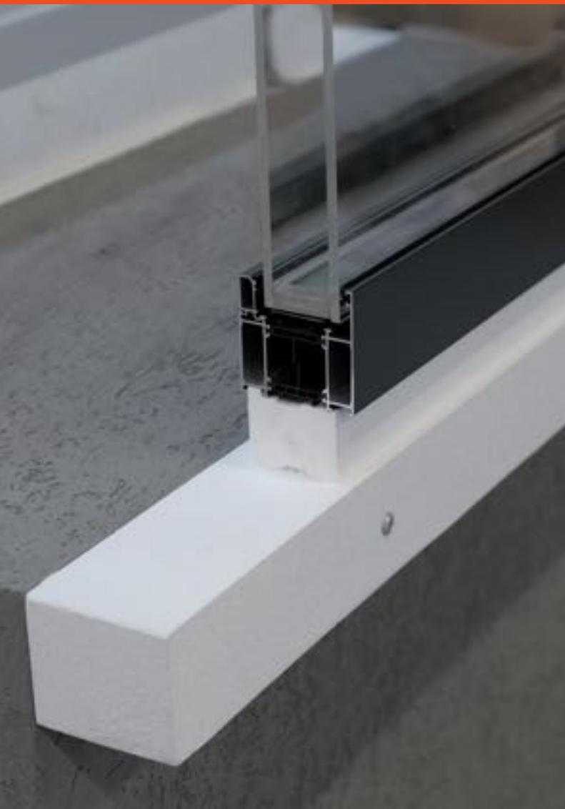
With the COMPACFOAM Frame Support system, windows and doors can be installed in the external insulation layer and avoid thermal bridges. This means that the windows and doors are installed beyond the solid outer walls into the external wall thermal insulation. This method is known as pre-wall mounting.
